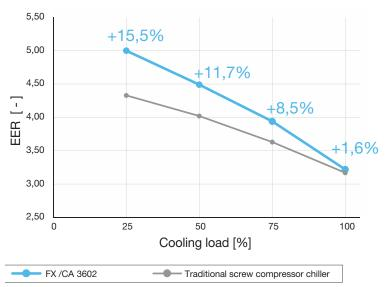
) graph shows the chiller efficiency with the variation of the load rate and air temperature (ESEER operating conditions
