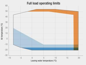
The diagram shows the operating limits of versions /E, /SL-E For versions /K, /SL-K, the max outdoor temperature is lowered by  $4^{\circ}$ C
