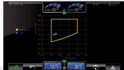
The interface allows for easy unit intervention (the safe access to data is ensured by three different password levels), and the graphic display of the monitored values. A dedicated section for the trouble shooting is also available.
