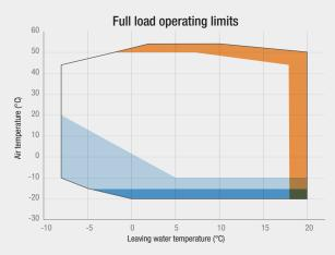
The diagram shows the operating limits of versions /E, /SL-E For versions /K, /SL-K, the max outdoor temperature is lowered by  $4^{\circ}\text{C}$
