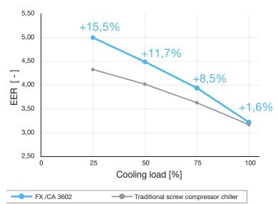
3 graph shows the chiller efficiency with the variation of the load rate and air temperature (ESEER operating conditions
